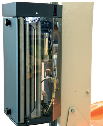
OSCAR TOUCH V.5 Film tensioning with motorized pre-stretch
