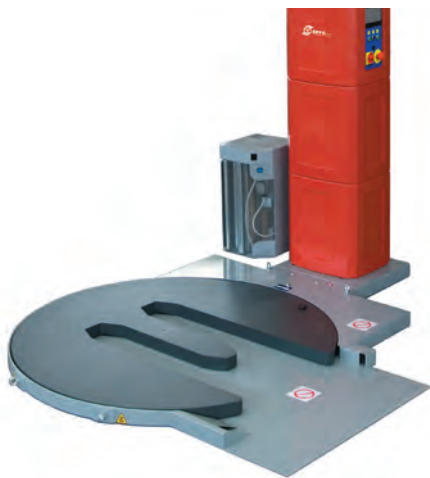
TP ROTARY TABLE SHAPED FOR PALLET TRUCK FORK ENTRY
